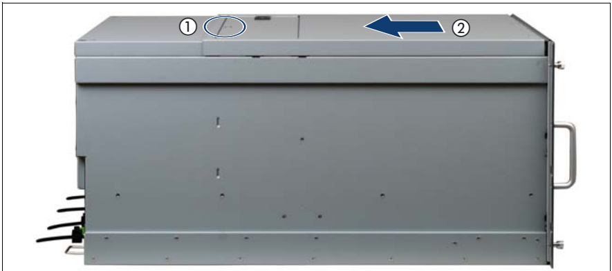
Figure 6: Removing the front cover
